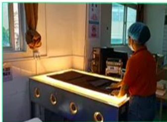
Power output testing for finished product
