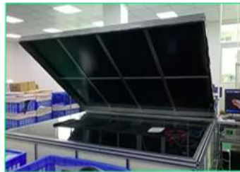
EL testing for foldable solar panel
